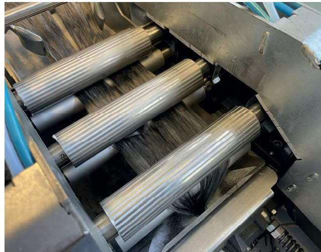
Fig. 5: Illustration of coated drafting system rollers integrated into the drafting system with elastic base layer and segmented surface, used for the processing of a hybrid carding tape made from recycled carbon fibers and thermoplastic fibers.
